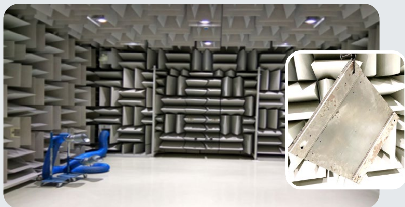
Figure 10: Point mobility test in anechoic chamber captured shifting of peaks to higher frequencies and significant reduction of amplitude responses of spot-welded and bonded floor section with elastic rubber-based hem-flange adhesive.
