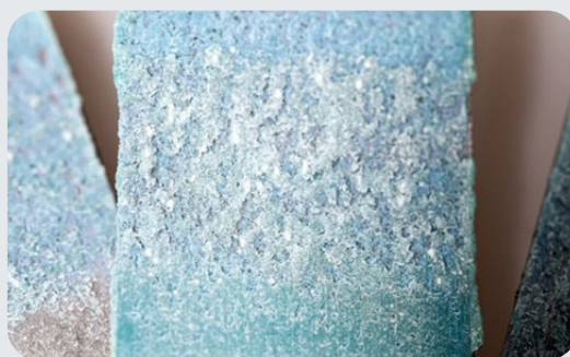
Figure 11: Lap shear and impact peel testing with Henkel TEROSON adhesives showing 100% cohesive failure.
