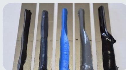
Figure 7: Bathing process of car body (left picture). Rotating Immersion method used to prove the Wash-Off resistant of Henkel adhesives. These wash-off test samples show good bead stability via control over yield point and thixotropy (right picture).
