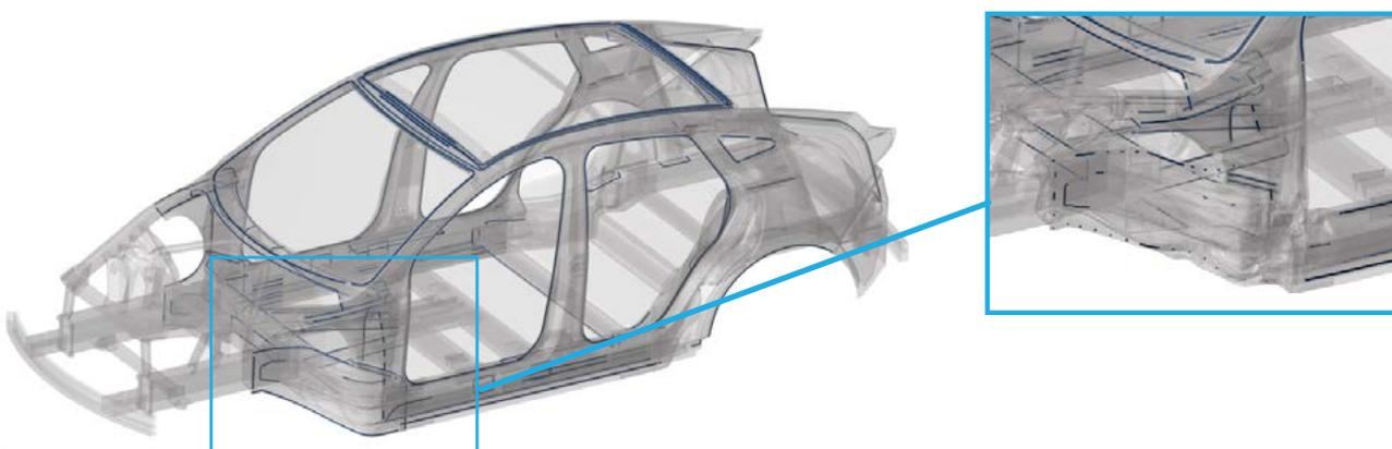
Figure 13: Failure prediction of high crash-resistant structural adhesive in BIW in IIHS small overlap crash
