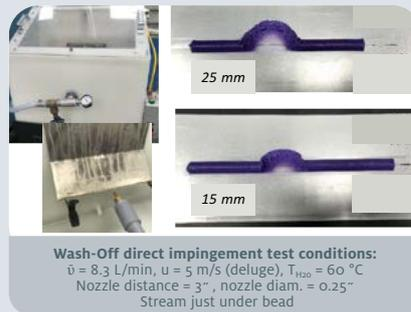
Figure 9: BIW goes through e-coat bath process (left picture) and an example of wash-off resistance test according to GM specific direct impingement test on various bead widths (right pictures)
