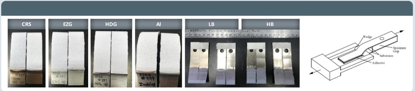
Figure 7: Cohesive-type failures after T-Peel test on Cold Rolled Steel (CRS), Electro Zinc Galvanized (EZG) steel and Hot Dip Galvanized (HDG) steel and Aluminum substrates also after IWP test cured at low (LB) and high bake (HB) temperatures
