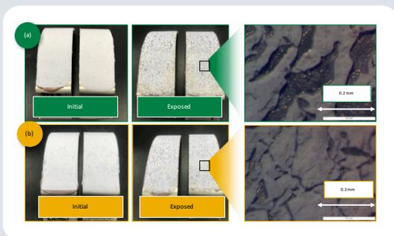
Figure 10: (a) Initial and (b) optimized reduction of blistering and interfacial failure due to moisture absorption
