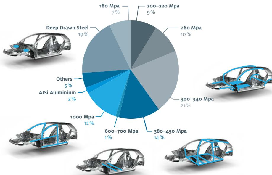
Figure 1: BIW material distribution (Baron et al. Assessing the Fleet-wide Material Technology and Costs to Lightweight Vehicles. CAR 2016)
