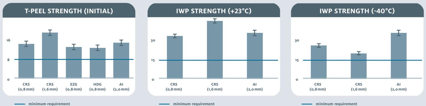
Figure 6: T-Peel and IWP strengths of typical crash-resistant structural adhesive on Cold Rolled Steel (CRS), Electro Zinc Galvanized (EZG) steel and Hot Dip Galvanized (HDG) steel and Aluminum substrates with various thicknesses
