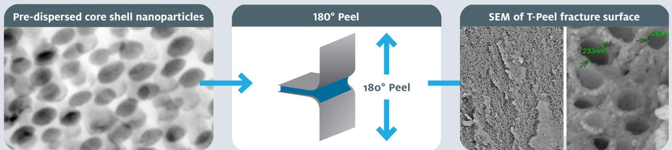
Figure 5: Toughening effect of pre-dispersed rubber nanoparticles on T-Peel fracture surface
