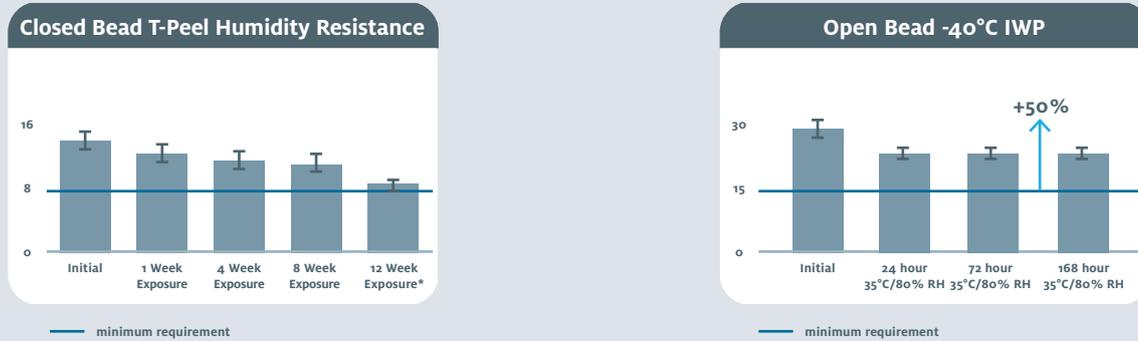
Figure 11: T-Peel and IWP at -40°C strengths after humidity exposure on open and closed beads (\*: 3 months uncured exposure 35°C at 85% RH)
