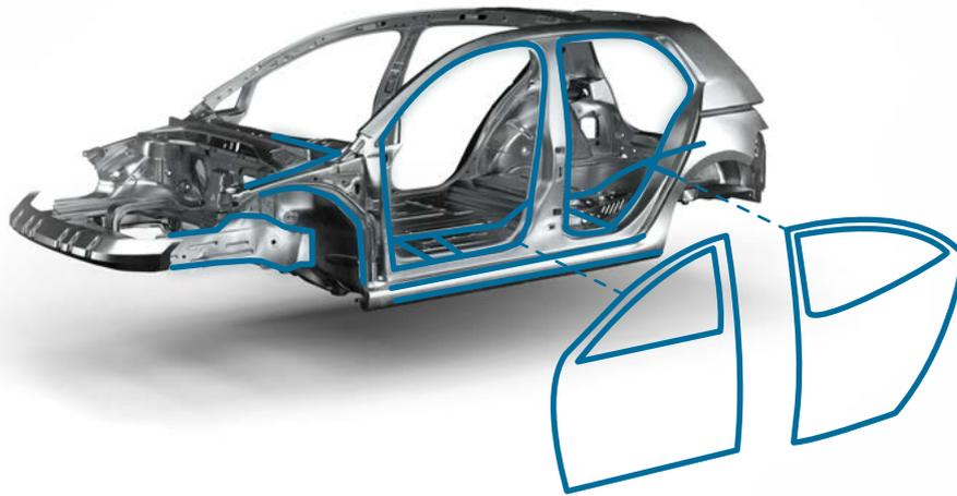
Figure 3: High crash-resistant structural adhesive typical application locations
