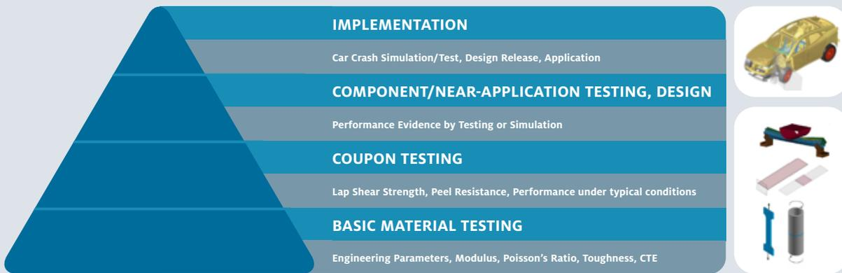
Figure 12: Engineering process from generating, validating and final implementation of simulation material data input of Henkel's structural adhesives
