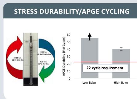
Figure 8: APGE environmental cycling for stress durability test according to ISO 11343 test method
