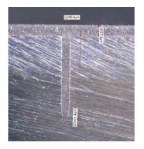
A trench measuring 40  $\mu m$  in width by 400  $\mu m$  in depth is completely filled with no voids using the next-generation LCM material.
