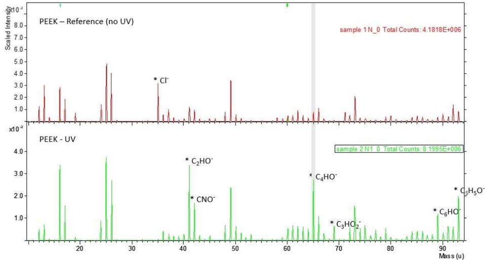
Figure 3. TOF-SIMS spectrum diagrams of PEEK panels before and after UV pretreatment.
