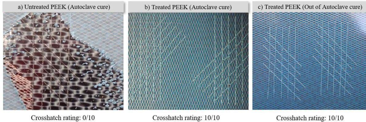
Figure 11. Effect of pretreatment on bonding of surfacing film to PEEK composite panels: Inside and out of autoclave cured at 177 °C.
