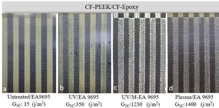
Figure 6. Adhesive bond failure mode of DCB specimen a) untreated/EA 9695, b) UV/EA9695, c) UV/Modified (M)-EA 9695, d) Plasma/EA9695. The thermoplastic and thermoset strip from each DCB specimen are paired where the black 5HS woven pattern strip is PEEK.
