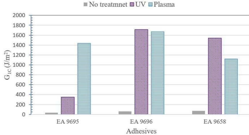
Figure 4. Fracture toughness ( $G_{1C}$ ) measurements of PEEK samples bonded with EA 9696, EA 9695, and EA 9658 with and without UV and plasma pretreatment.
