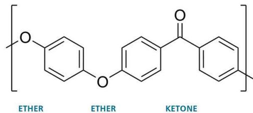
Figure 1. Chemical structure of PEEK.
