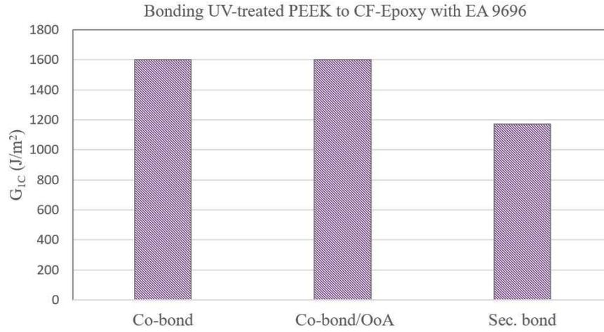
Figure 7. Comparing different bonding of UV treated PEEK to CF-Epoxy
