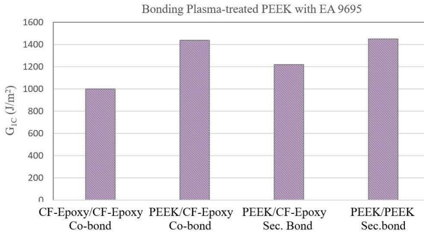
Figure 8. Comparing different bonding of Plasma treated PEEK to CF-Epoxy
