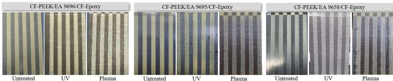
Figure 5. Adhesive bond failure mode of DCB specimens with and without UV and plasma pretreatment. The thermoplastic and thermoset strip from each DCB specimen are paired where the black 5HS woven pattern strip is PEEK.
