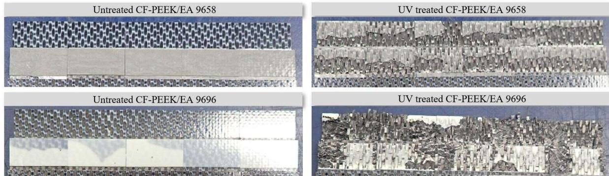
Figure 10. Adhesive bond failure mode of notched tensile lap shear specimens with and without UV treatment.
