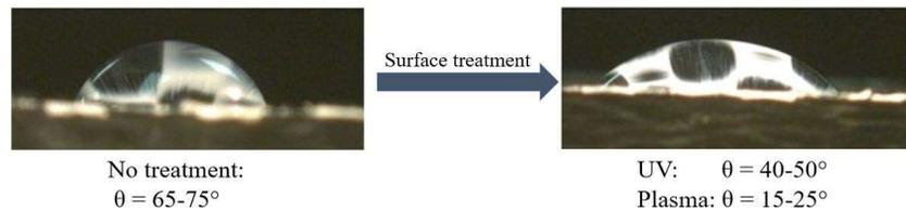
Figure 2. Contact angle ( $\theta$ ) of a water droplet on PEEK panel surface before and after surface pretreatment.
