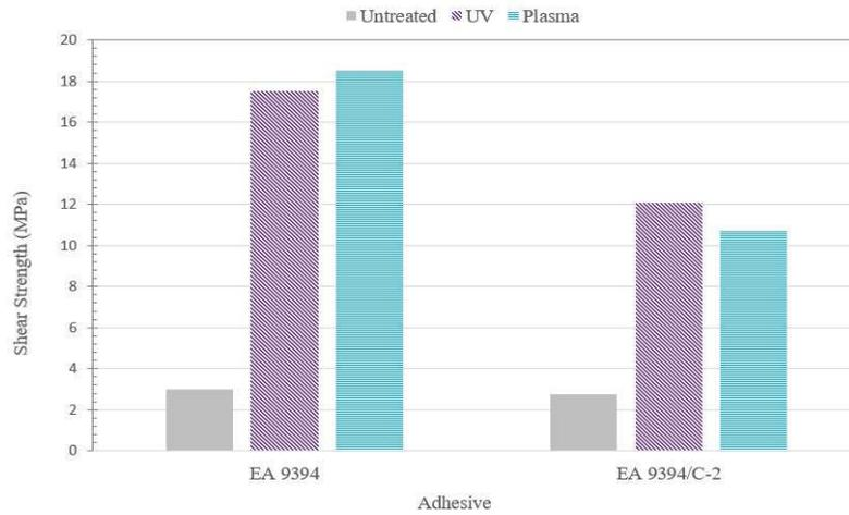
Figure 9. Tensile lap shear of PEEK substrates bonded with a room-temperature cure (EA 9394) and an elevated-temperature cure (EA 9394/C-2) paste adhesive with and without pretreatments
