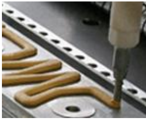
Figure 9. Dispensed Bead of Liquid Paste
