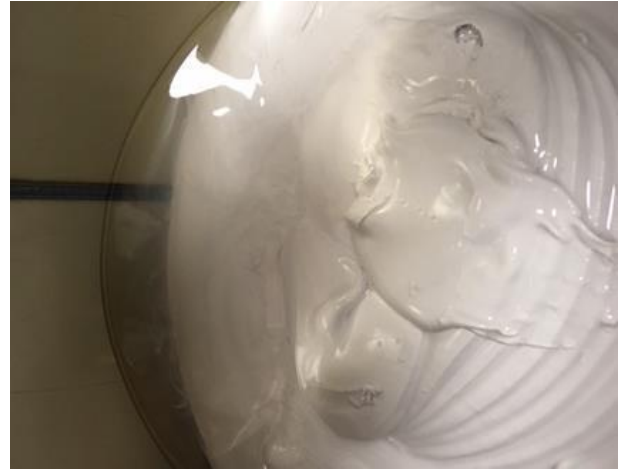
Figure 15. Separation in a TIM Material
