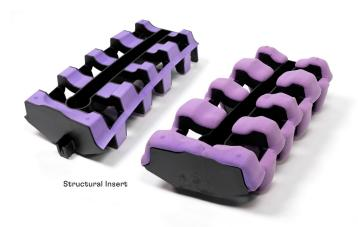
**TEROSON EP 1475** offers superior compression strength for excellent crash performance, with up to a 300% expansion rate for large gap-filling capability. For slower-heating areas of the body-in-white, TEROSON EP 1475 cures at 140°C in 10 minutes
