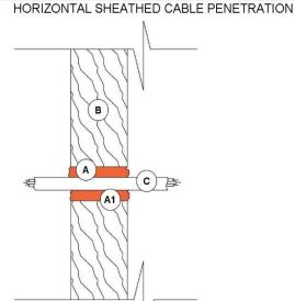
A and A1: OSI Fire Block Foam applied between gap at vertical framing and horizontal penetration material. Gap between framing and penetration material must be a minimum of a 1/4" inch. Fire Block Foam must fill gap. Do not cut expanded foam after cure.
