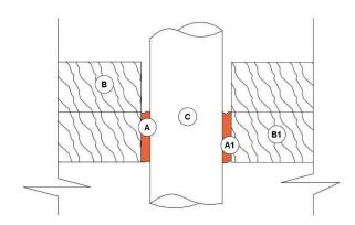
**A and A1:** OSI Fire Block Foam applied between gap at horizontal double top plate framing and vertical pipe. Gap between framing and penetration material must be a minimum of a 1/4" inch. Fire Block Foam must fill gap. Do not cut expanded foam after cure.
