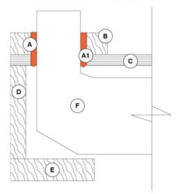
A and A1: OSI Fire Block Foam applied between gap at horizontal bottom wall plate framing and vertical penetration material. Gap between framing and penetration material must be a minimum of a 1/4" inch. Fire Block Foam must fill gap. Do not cut expanded foam after cure.
