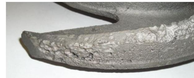
Worn impeller prior to repair.
