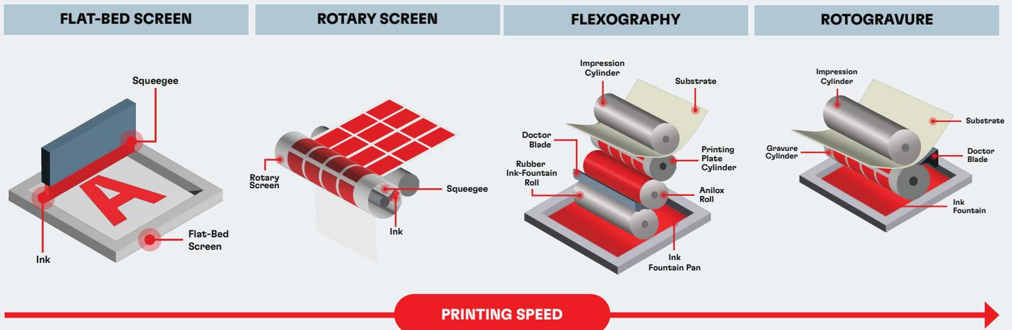
The advantage of screen printing is the ability to apply thick layers (5 - 25  $\mu\text{m}$ ), but it is a slower process in comparison with flexographic or gravure printing.
