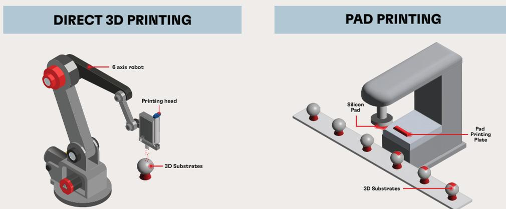
Pad-printable functional inks allow customers to print directly onto 3D-shaped surfaces, eliminating the need for wires, etching, or electroplating. Direct 3D printing is enabled by placing a printing head at the end of a robotic arm. The print head can be adjusted to different coating processes, such as spray-coating, valve-jet dispensing, aerosol jet, and dispensing.
