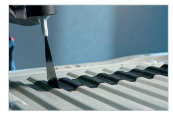
ACOUSTIC BEADS Reproduction of wdestream beads for reduction of vibration borne noise.
