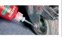
Very difficult to disassemble with standard hand tools; may require localised heat for removal. For preassembled fasteners, instrumentation or carburettor screws.
