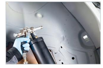
ACOUSTIC COATING Application of stone chip coating for reduction of vibration borne noise.
