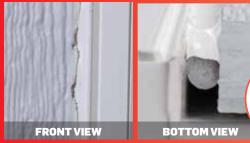
• Dimension C beyond standard maximum depth. This will debilitate joint movement capability causing fissures and fractures • Slow cure due to excessive sealant depth may compromise sealant performance • Dimension B beyond standard maximum depth
