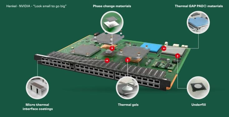
materials are used throughout a circuit board configuration and help optimize performance of the electronic components that house them—such as AAUs, routers, switches, and servers.
