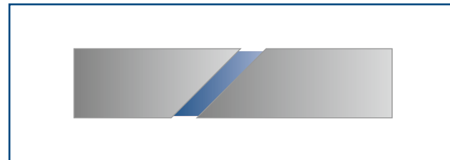
SCARF JOINT: A scarf joint is an angular butt joint. Cutting the joint at an angle increases the surface area.
