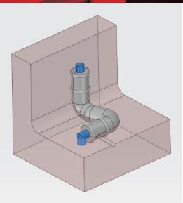
Parts were 3D printed at a cost of \$19 each – a far cry from the \$190 per part quoted for injection molding.
