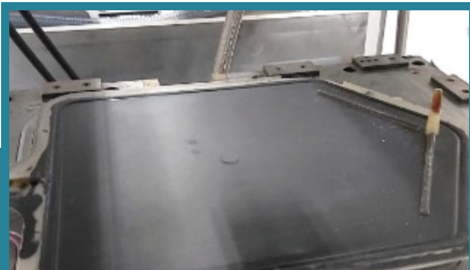
FIGURE 4: Panel made from HP-RTM Process with AMRC and Henkel's LOCTITE RI 9501 AERO.
