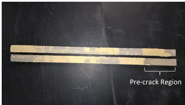
Figure 15. Dual Cantilever Unfilled Resin 2 Failure Surface
