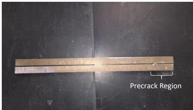
Figure 15. Dual Cantilever Unfilled Resin 2 Failure Surface
