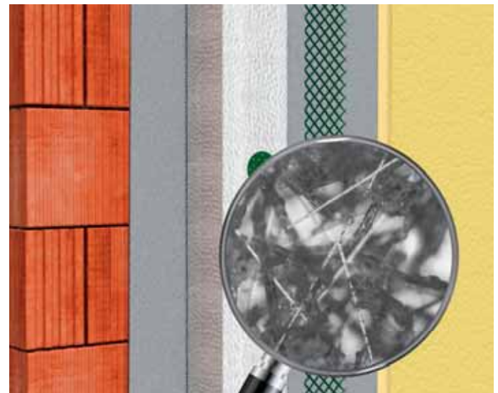
ETICS system with focus on rendering mortar strengthened with Fibre Force unique fibres combination.
