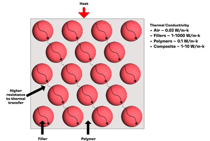
Illustration of filler in a polymer matrix.
