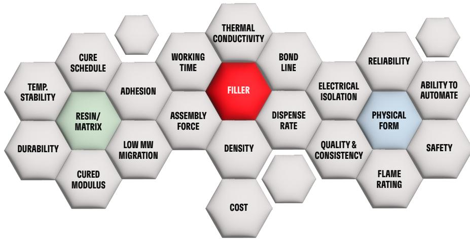
Illustration of key building blocks for TIMs that determine final performance, handling, and format of the material.
