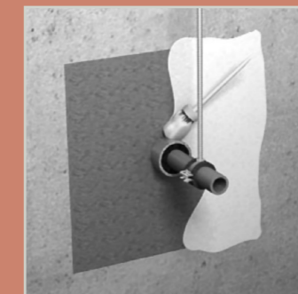
Final coating on FP 550 foam. Used as a system component for all penetration seals.
