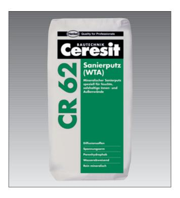
Prepare pneumatic mortar of a suitable consistency using CR 62 mixed with CC 81 and water (mixing ratio: CC 81: water = 1:3) and throw onto the wall. Apply the mortar in a net-like pattern with only 50% coverage. With mixed brickwork, porous bricks and sand-lime bricks apply the mortar with at least 5 mm layer thickness.
