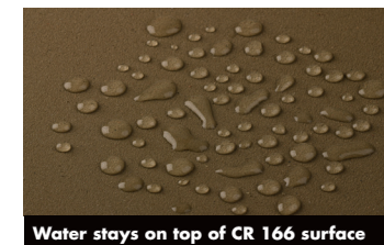
Water stays on top of CR 166 surface
