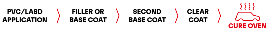
Optimal 1-Oven 4Wet "4-Coat 1-Bake" Process (up to 5kg additional CO 2 saved* per vehicle processed)
