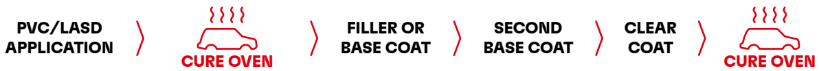
Intermediate 2-Oven 3Wet Curing Process (up to 5kg CO 2 saved* per vehicle processed)
