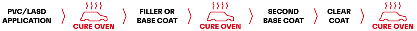
Traditional 3-Oven Paint Shop Curing Process (up to 15kg CO 2 generated per vehicle processed)
