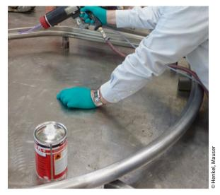
Figure 3 > Cleaning of the flanges
