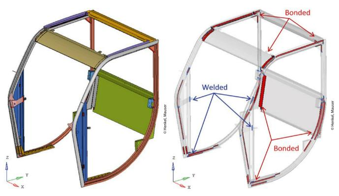
Figure 1 > CAD model of the cabin frame
