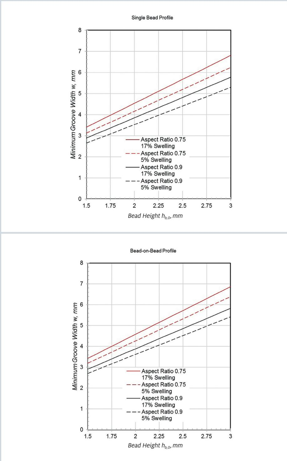
Figure 22: Minimum groove width corresponding to a bead deformed by 45% compression and immersed in oil at 150°C.
