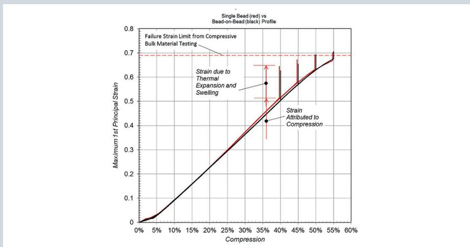
Figure 19: Compression-strain curves for bead profiles at different compression levels for both single bead and bead-on-bead, shown in red and black, respectively. The total strain resulting of compression and thermal expansion/swelling exceeds the failure limit of the material, leading to failure at compression level above 45%.
