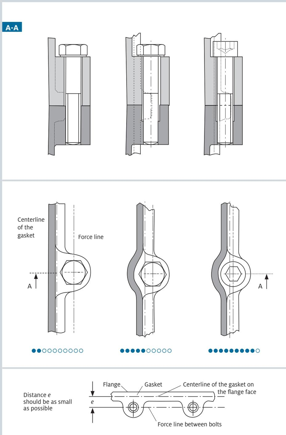
Figure 5: Evaluation of the distance between bolt force lines and centerline of the gasket in regard to the compressive stress distribution in the seal gap<sup>1</sup>.
