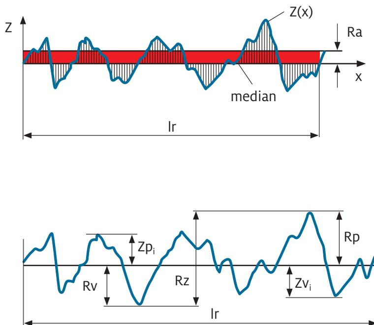
Figure 10: Ra and Rz according to DIN EN ISO 4287.
