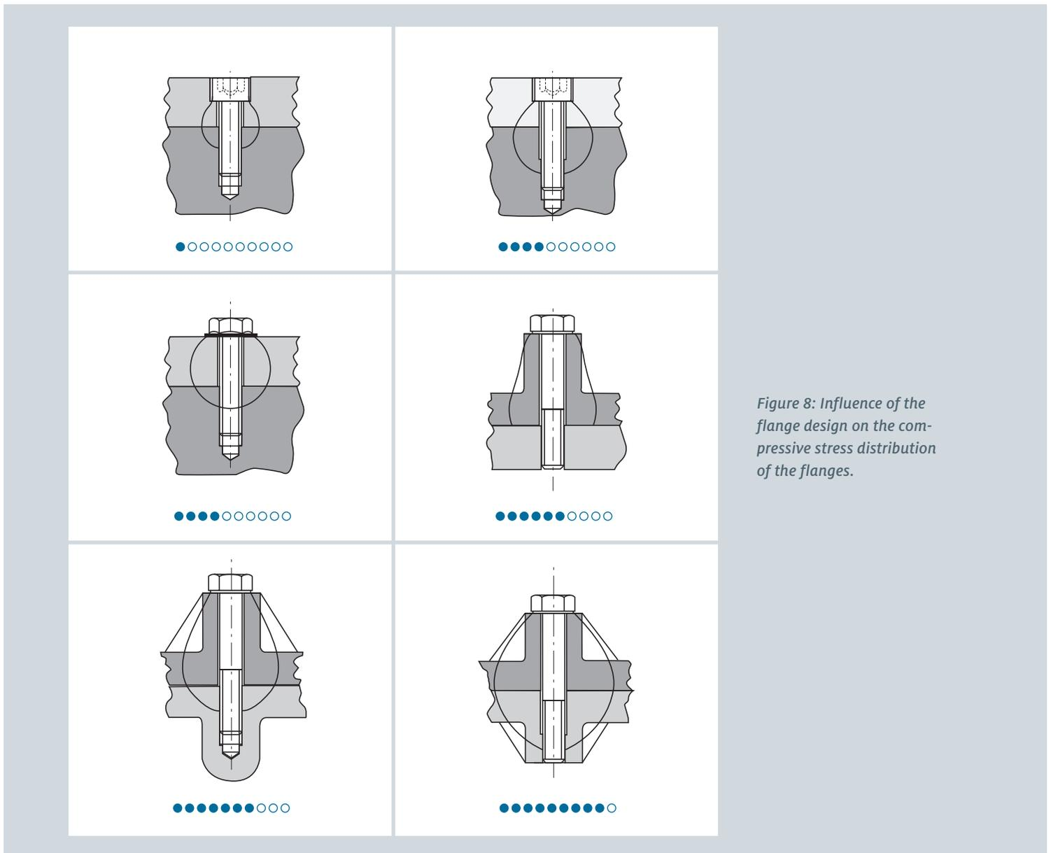
Figure 8: Influence of the flange design on the compressive stress distribution of the flanges.
