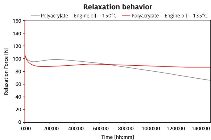
Compression set is the term, which describes the loss of elastic memory of the elastomer, the better the elastomeric memory the lower the compression set.
