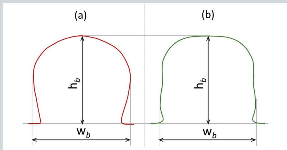
Design rules and recommendations address the issues of purposeful compression and space needed for a groove or step to house the bead and provide adequate void volume for the flow of the material in compression. They are based upon functional experiments, material testing, and numerical analysis results.
