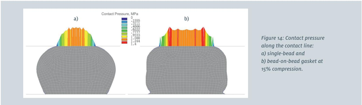
Figure 14: Contact pressure along the contact line: a) single-bead and b) bead-on-bead gasket at 15% compression.
