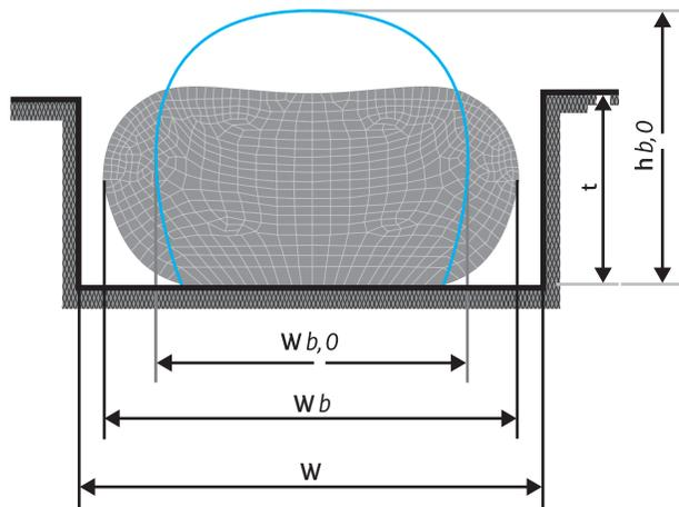
Based upon numerical simulations, the expected width of the bead under assembly conditions,  $w_b$ , may be estimated with significant accuracy. Its value corresponds to a minimum required groove width, which has to be appropriately enlarged by a safety factor for design purposes. The estimated width takes into account both deformation due to compression after assembly and expansion due to thermal loading and swelling (figure 21).
