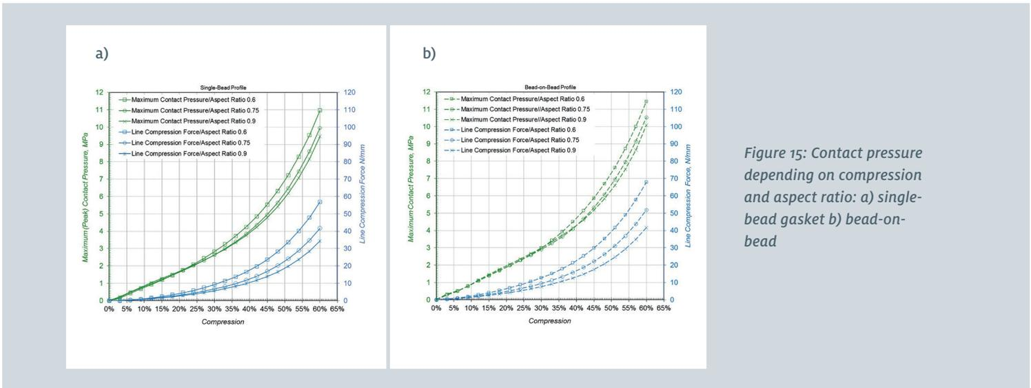
Figure 15: Contact pressure depending on compression and aspect ratio: a) single-bead gasket b) bead-on-bead
