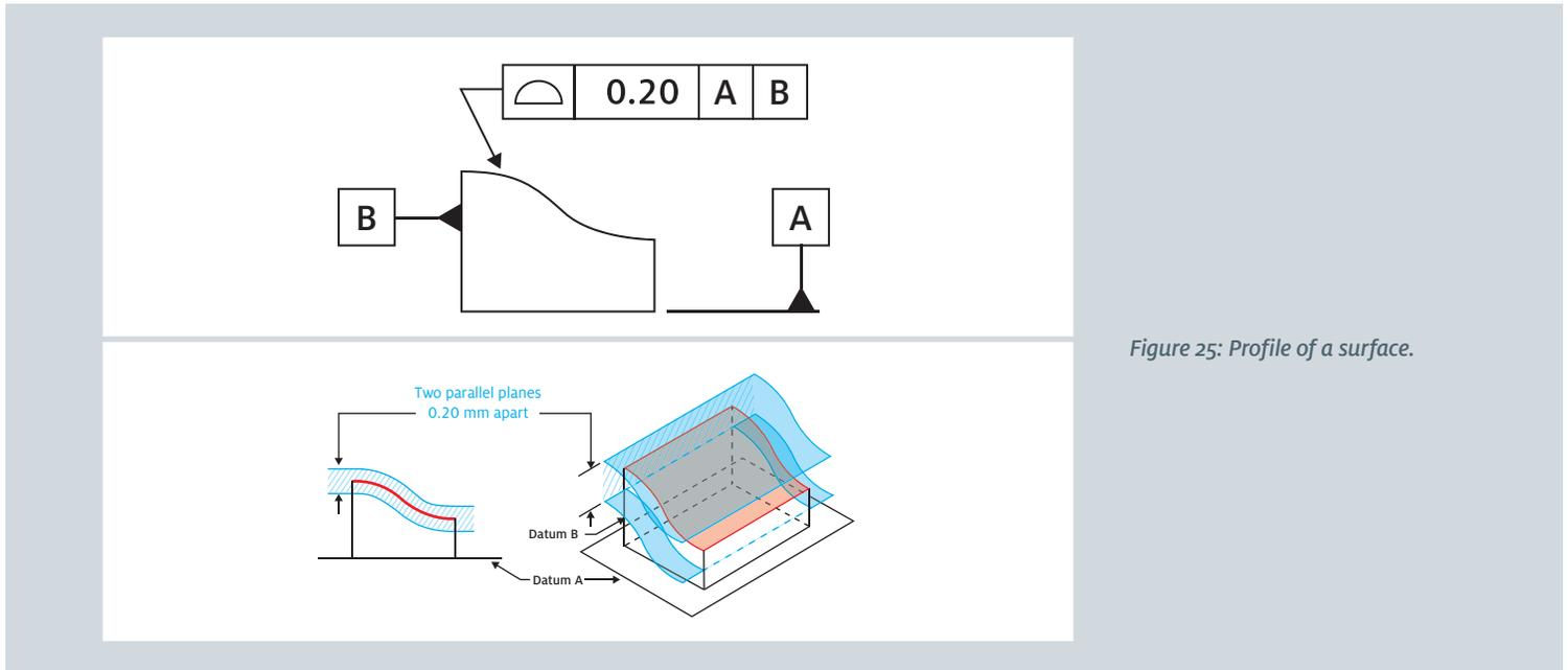
Figure 25: Profile of a surface.
