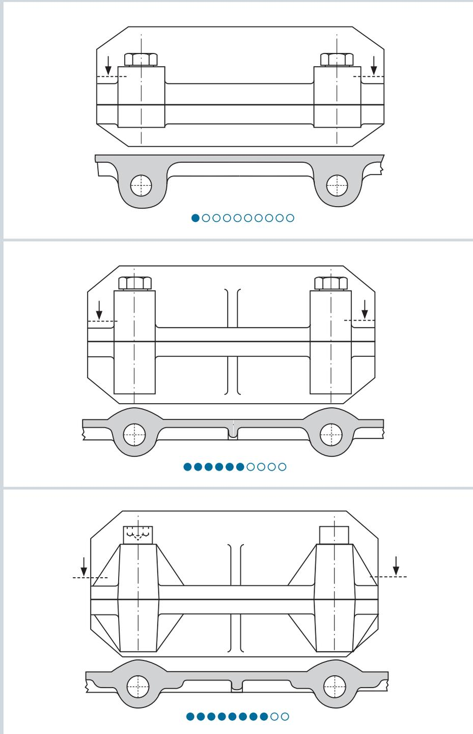
As flange rigidity decreases, the more complicated it will be to obtain the required minimum surface pressure at midpoint between two bolts.
