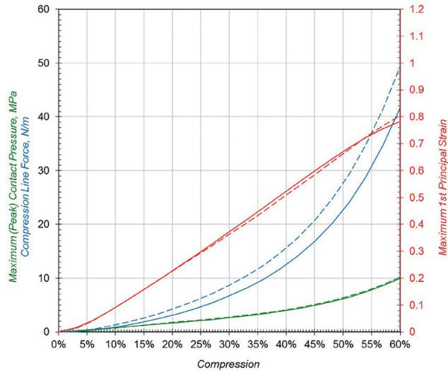
The minimum compression level for retaining sealability is 15% for both single and bead-on-bead designs. This value was validated by testing gaskets immersed into oil under thermal cyclic loading conditions (figure 17).
