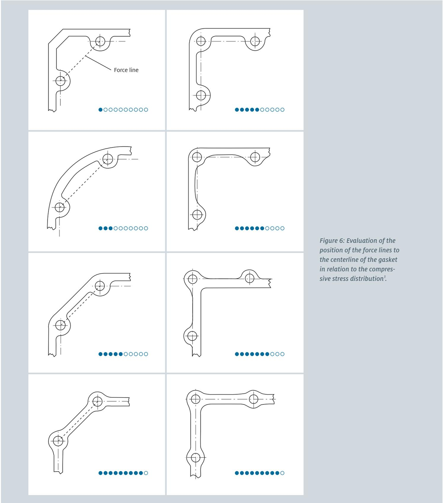
Figure 6: Evaluation of the position of the force lines to the centerline of the gasket in relation to the compressive stress distribution<sup>1</sup>.
