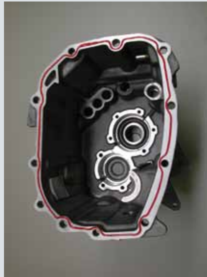
Figure 19: Anaerobic product bead on gearbox flange.
