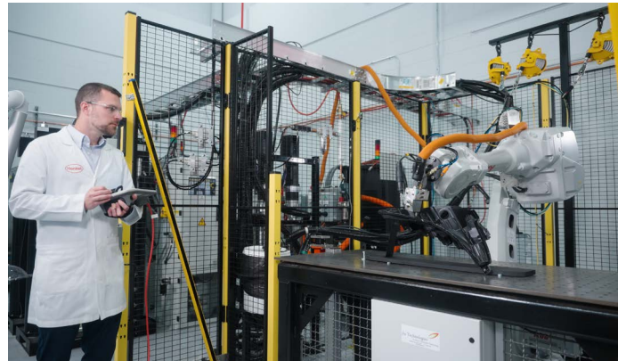
Six-Axis ABB Robot for Automated Dispensing: Interchangeable Dispense Heads
