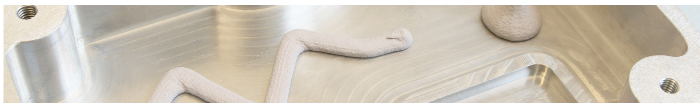
Cured-in-place gasketing material
