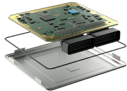
GAP PAD material on Electronic Control Unit
