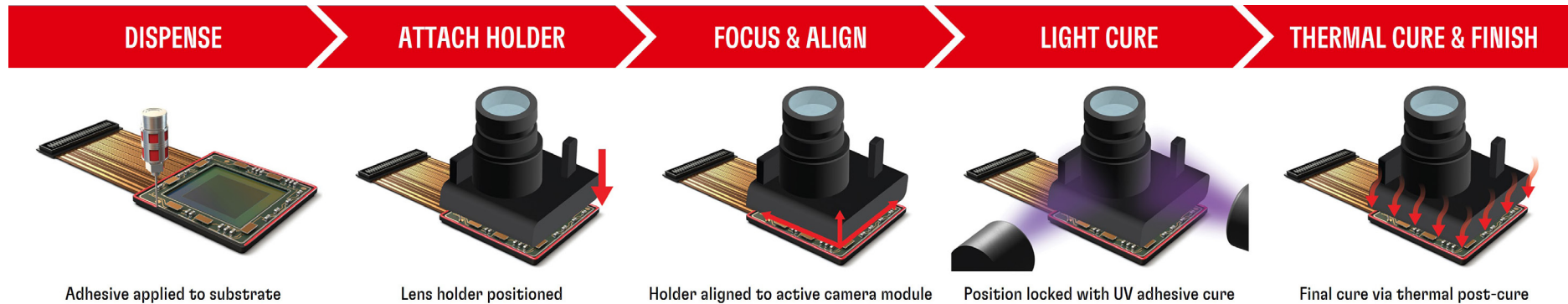
Figure 2. Typical active alignment steps in ADAS camera module assembly.
