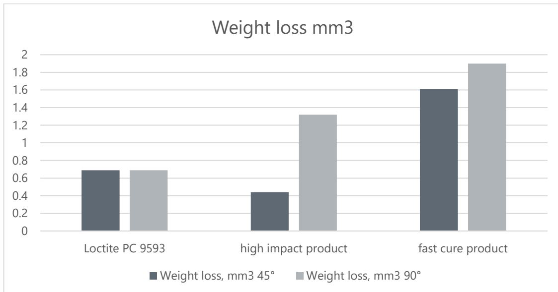
FIGURE 5. Volume loss results from gas jet erosion test.
