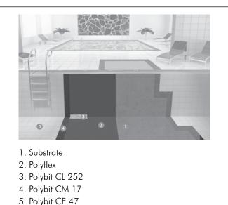
Joint filing of the tiles is done with Polybit CE 47 chemical resistant epoxy resin based joint filling grout.
