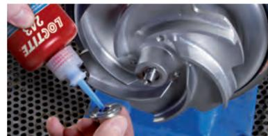
Difficult to disassemble with standard hand tools good for permanent assemblies for thread size up to M50.
