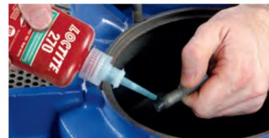
Very difficult to disassemble with standard hand tools; may require localised heat for removal good for permanent assemblies at heavy equipment, studs, motor and pump mounts, for thread size up to M50.
