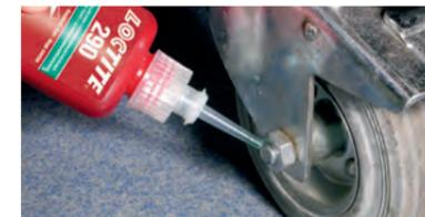
Very difficult to disassemble with standard hand tools; may require localised heat for removal. For preassembled fasteners, instrumentation or carburettor screws.
