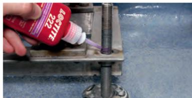
Removable with standard hand tools, good for adjustment screws, calibration screws, meters and gauges, for thread size up to M36.
