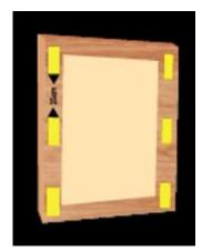
Apply strips without air-bubbles to the substrate and remove yellow protective liner. Press item to be bonded firmly into place. Support heavier items for 24 hours.
