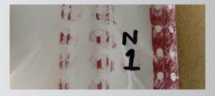
The example shows an adhesive pattern outside of the intended vacuum pad area.
