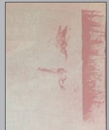
Figure 1 Poor slot die application
