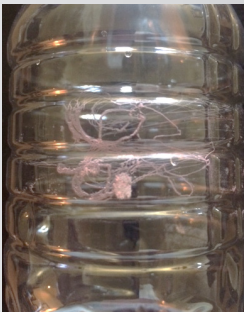
Example of a non-optimized spray application. Spirals are not uniform and may “blow” outside the label.
