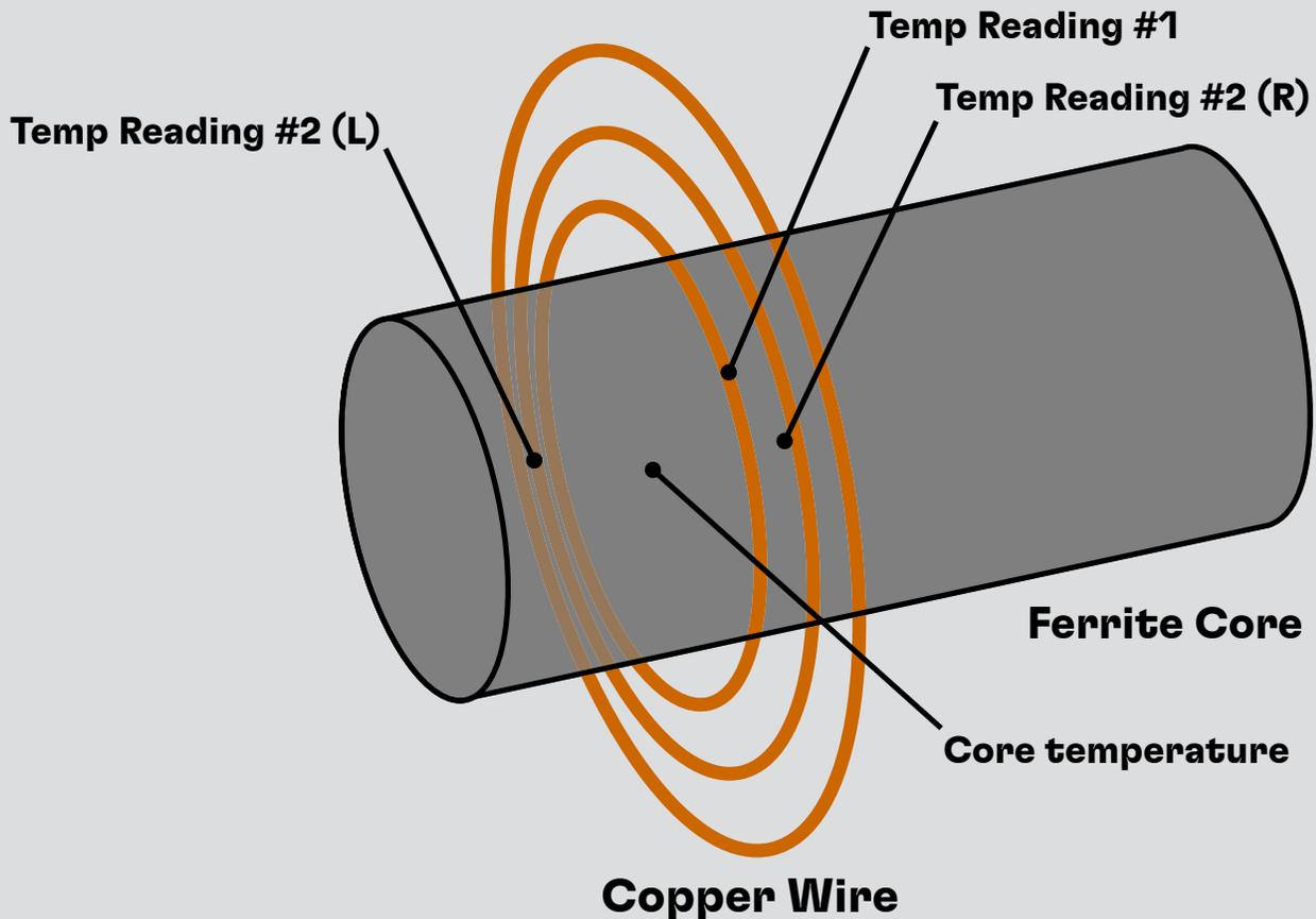
A constant load was applied to the potted component and the steady state temperature was measured at the three different points. Despite a lower nominal thermal conductivity, LOCTITE SI 5643 provided both lower average temperature and better homogeneity in this applied test, which shows how it is important to look beyond the data sheet for potting applications.
