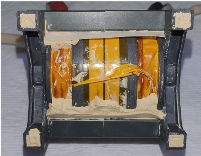
Figure 3: Ferrite Core Remained Intact
