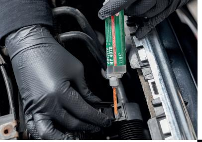
Application of the adhesiveApply LOCTITE HY 4070 to the repair area.
