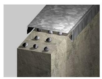
After assembly, the thickness of the adhesive strand must be  $\geq$  1mm. If necessary, use spacers. The application temperature must be between -5 °C and +40 °C. Heavy workpieces or pieces under tension must be supported or fixed if necessary.
