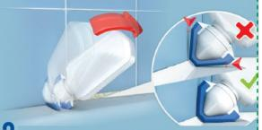
Place nozzle on sealant with Pattex Logo facing you, tilt to ensure a tight seal between the wall/bath, shower or sink
