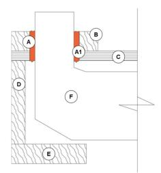
A and A1: Pro Gaps & Cracks Foam applied between gap at horizontal bottom wall plate framing and vertical penetration material. Gap between framing and penetration material must be a minimum of a ¼". Pro Gaps & Cracks Foam must fill gap. Do not cut expanded foam after cure.
