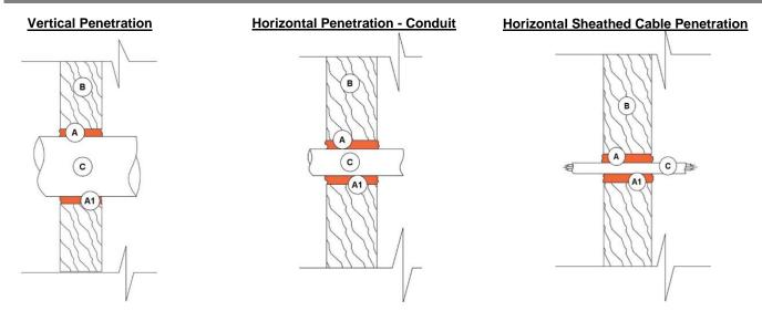
A and A1: Pro Gaps & Cracks Foam applied between gap at vertical framing and horizontal penetration material. Gap between framing and penetration material must be a minimum of 1/4". Pro Gaps & Cracks Foam must fill gap. Do not cut expanded foam after cure.
