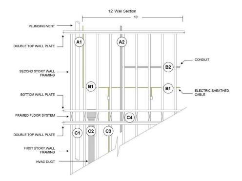
A1: PVC plumbing vent and electric sheathed cable at vertical penetration at ceiling level, trough double top plate, must be sealed with fire block foam
