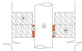
**A and A1:** Fire Block Foam applied between gap at horizontal double top plate framing and vertical pipe. Gap between framing and penetration material must be a minimum of ½" (6 mm). Fire Block Foam must fill gap. Do not cut expanded foam after cure.
