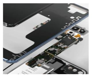
Henkel's PDS antenna technology enables design flexibility to replace incumbent antenna solutions for smaller space
