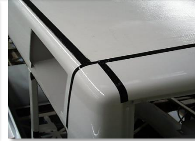
Sealing GRP and metal parts on roof elements
