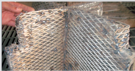
Splitter section of burner tip with spot-welded wire mesh. Ready of PC-7000™ coating
