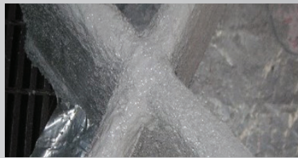
Burner tip splitter coated with PC 7000™
