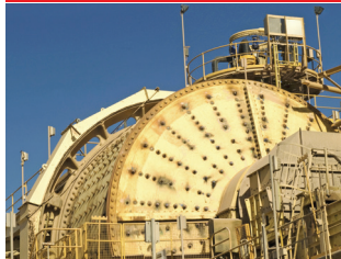
Ball Mill Trunnions & Feed Chutes
