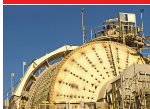
Ball Mill Trunnions & Feed Chutes
