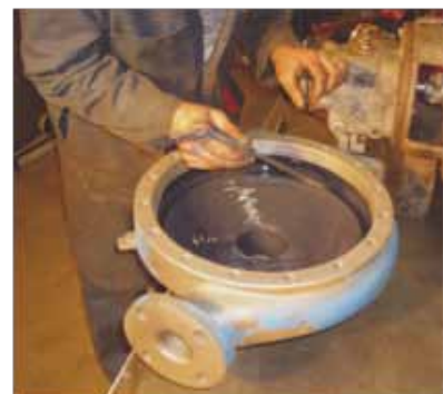
LOCTITE® PC 7333 & LOCTITE® PC 7315 provides a high gloss low friction coating.
