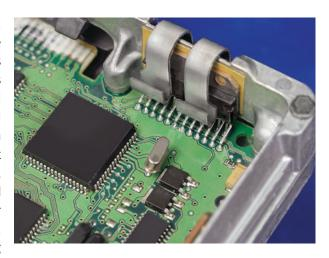
high-performance function of digital signal (DSP) and microcontroller (MCU) processors, as well as providing thermal relief from heat generation at the mid-frame. High conformity GAP PADs and automated, throughput-enhancing liquid form-in-place gap fillers effectively absorb and dissipate heat so radars can keep their cool.
