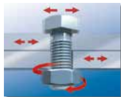
Vibration and loosening.
