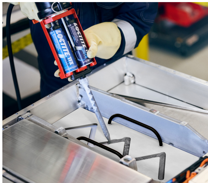
LOCTITE® TFX 3010 THERMAL GAP FILLER APPLICATION
